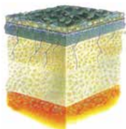
FibreDec used as a strain alleviating membrane (SAMI)
