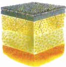
FibreDec surfacing over a cracked pavement wearing course (SAM)
