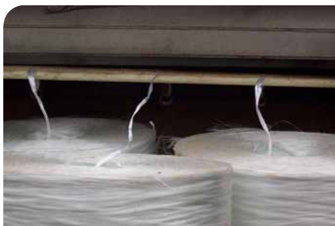
Rolls of glass fibre are fed into the FibreDec applicator box.
