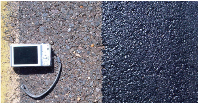
Side by side comparison of aged asphalt before and after JetBlack application.
