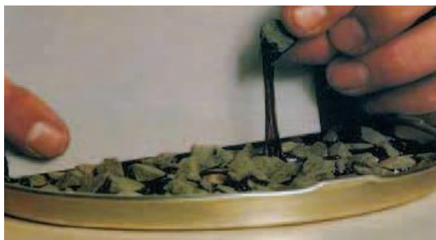
Surfix ® 70 emulsion exhibits excellent stone adhesion and torsional recovery.
