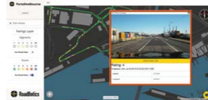
Port of Melbourne pavement condition data being displayed via RoadBotics web based portal Roadway.
