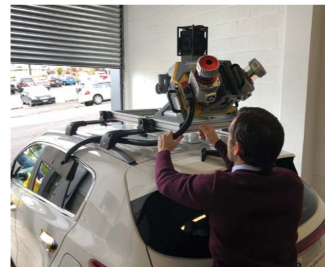
LiDAR with twin lasers linked to a 360 degree camera
