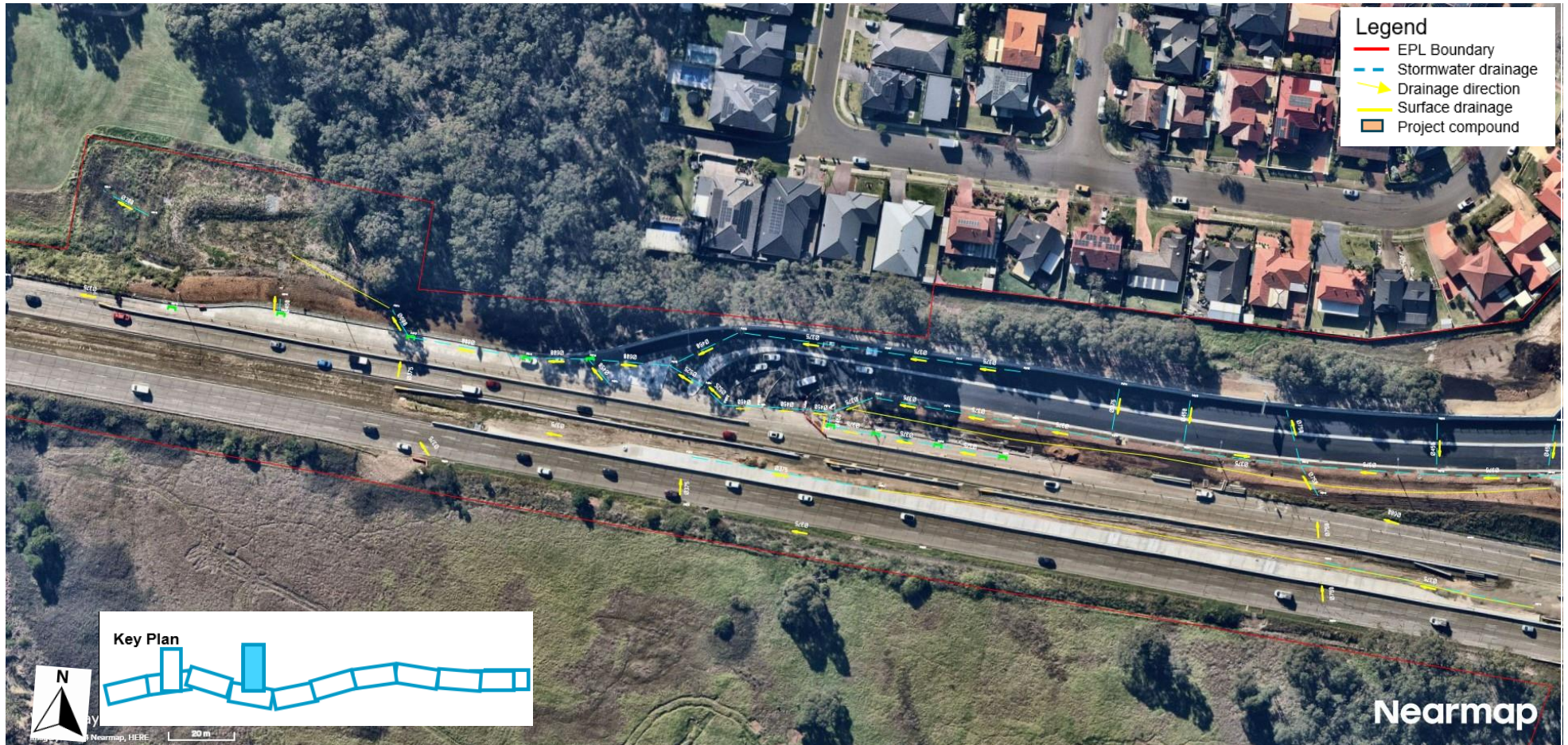
Figure 1: Project boundary and stormwater system
